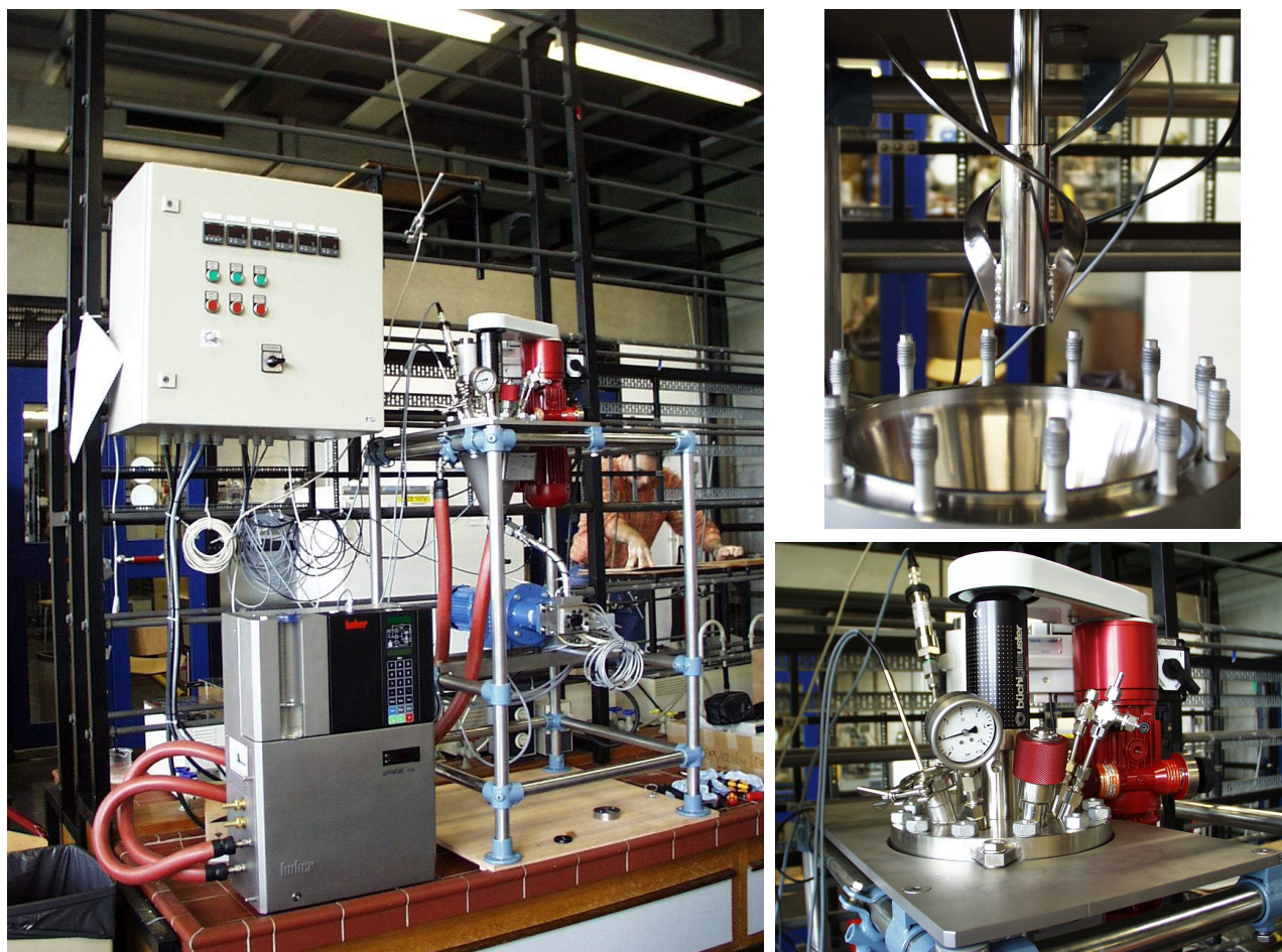
Figure 3.4 - 1 Kg scale synthesis unit. Left: overview. Top right: helical shaped stirrer. Bottom right: Cover plate of the reaction vessel, showing inlet valves and various sensors and the stirrer equipped with a 800 Ncm magnetic coupling fitted with a sensor for registering the torque. Next to the manometer is the connection for the condensor and cold trap (not shown). [Black and white figure on p. 41].
