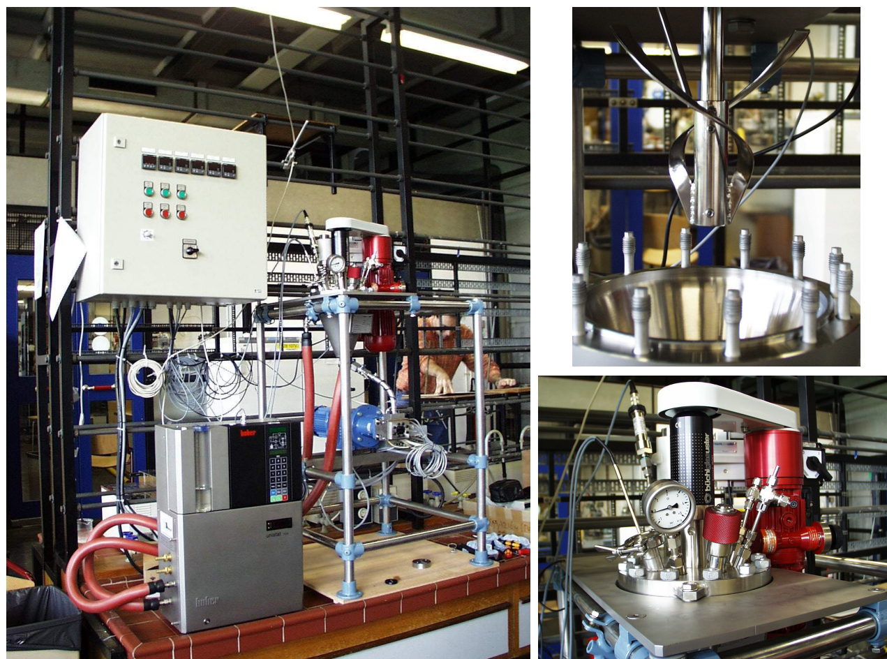
Figure 3.4 – 1 Kg scale synthesis unit. Left: overview. Top right: helical shaped stirrer. Bottom right: Cover plate of the reaction vessel, showing inlet valves and various sensors and the stirrer equipped with a 800 Ncm magnetic coupling fitted with a sensor for registering the torque. Next to the manometer is the connection for the condensor and cold trap (not shown). [Color figure on p. 168].
